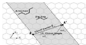
**Fig. 1: Illustration of how wrapping of graphite sheet form carbon nanotube [2]**
