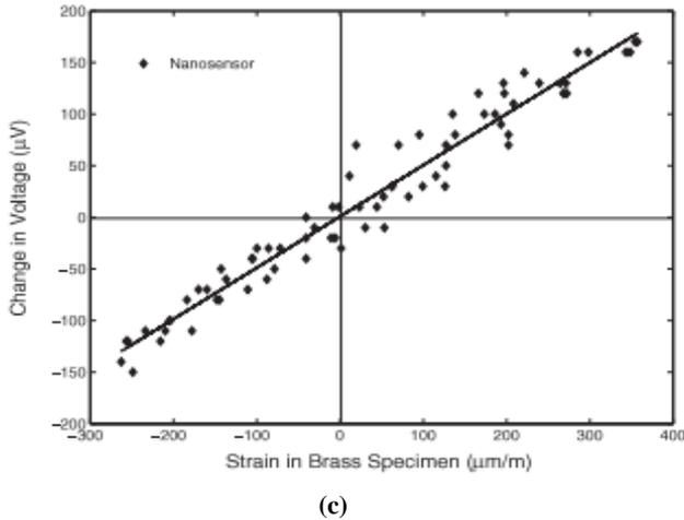
Fig. 4. (a) Picture of SBP film with insulating PVC attached to the brass specimen; (b) picture of metal strain gauge attached on the opposite side of the brass specimen; (c) Linear relationship between change in voltage in SBP film with respect to both tensile and compressive strain subjected to brass specimen [10].
